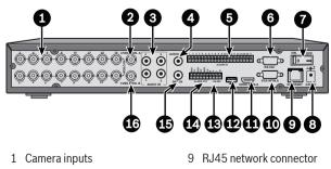
2 CVBS output - Monitor A 10 VGA output - Monitor A
