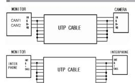
If you use UTP CABLE[CAT.5], connect the rest 4 lines to GND after connecting 4 lines between monitor and interphone.
