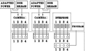
\* Each device should be connected by separated cables. If you use UTP CABLE[CAT.5] for CAMERA1and CAMERA2, 2 lines of UTP cable are required.
