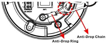
▲ NOTE: For safety concern, it is recommended to hook up the camera with the anti-drop chain of the pendant when installing the camera. For more information about pendant and anti-drop chain, please contact the camera manufacturer.
