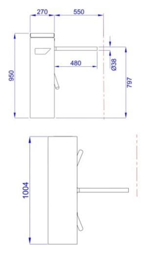
Important: Any horizontal pipe or conduit running below the Tripod Turnstile must be at least 140mm below FFL. Metal conduit for cables should be raised at least 50mm from foundation. It is the customer's responsibility to ensure the structural integrity and strength of the installation location. The dimensions given in this Product Data Sheet are for information only. In order to prepare the installation site, please refer to your usual Gunnebo Customer Service contact.
