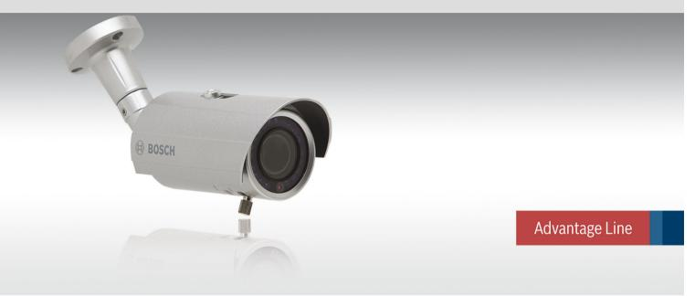
The WZ18 uses a 1/3 in CCD image sensor which delivers 540 TVL images. The 18 integrated infrared LEDs deliver 20 m (66 ft) of high performance night vision.
