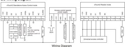
Note:Type A Electronic lock refers to the electric unlock when power on, such as electric control lock, electric lock. Type B Electronic lock refers to the electric unlock when power off, such as magnetic lock, electric bolt lock.
